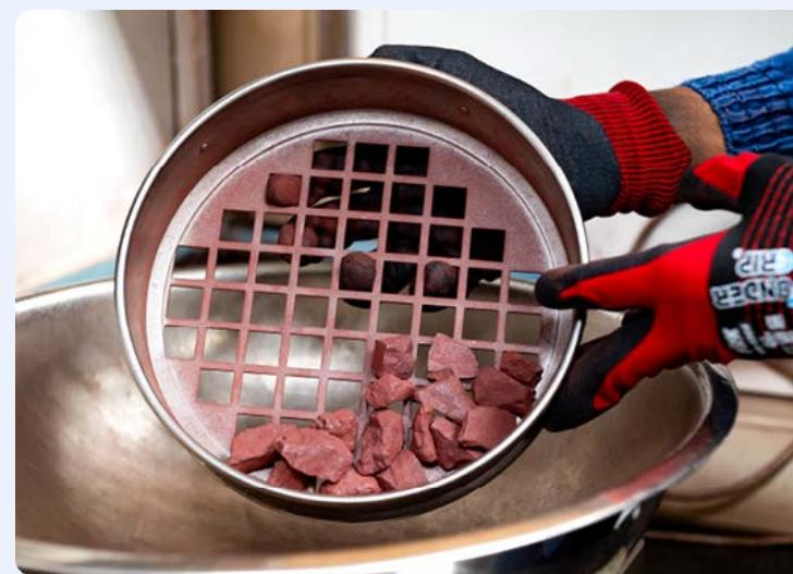
A sample of Kumba Iron Ore's DR Lump product after it has emerged from the screen plant, where the iron ore is reduced in size.
